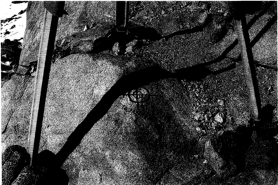
Plate 2. Top : theodolite station on ridge at western side of Gjelbreen. Bottom : reference point on firm ground, later provided with a cairn
